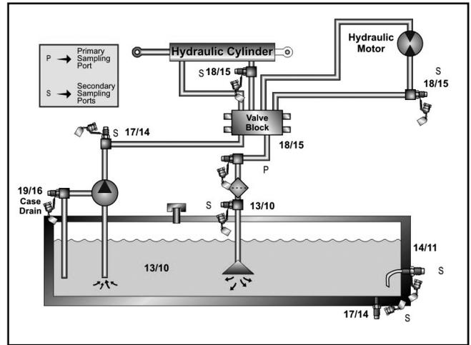
Figure 3: Sampling locations for a typical hydraulic system
