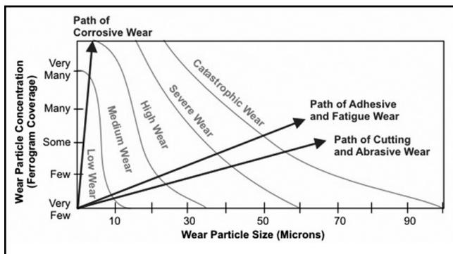
Figure 6: Particle size distribution for corrosive, cutting and adhesive wear
