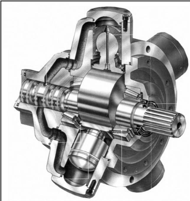
Figure 4: Radial Piston Pump. In this case, the portion of oil used to lubricate the bearings will exit back to the reservoir via the case drain.
