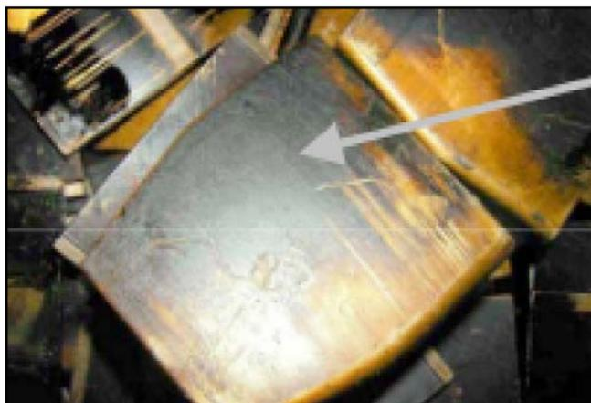
Figure 5: Gas turbine axial bearing pad deposit
